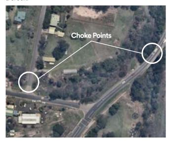
This customer found multiple fallen trees upstream of the bridge, mainly from the cause of recent fires that resulted in a lot of green waste debris. With significant rain, these trees could float downstream and become trapped within the choke point — creating a dam that causes water to flood into nearby homes and businesses. (One of the trees measured with Nearmap was found to be over 32 feet long.)
