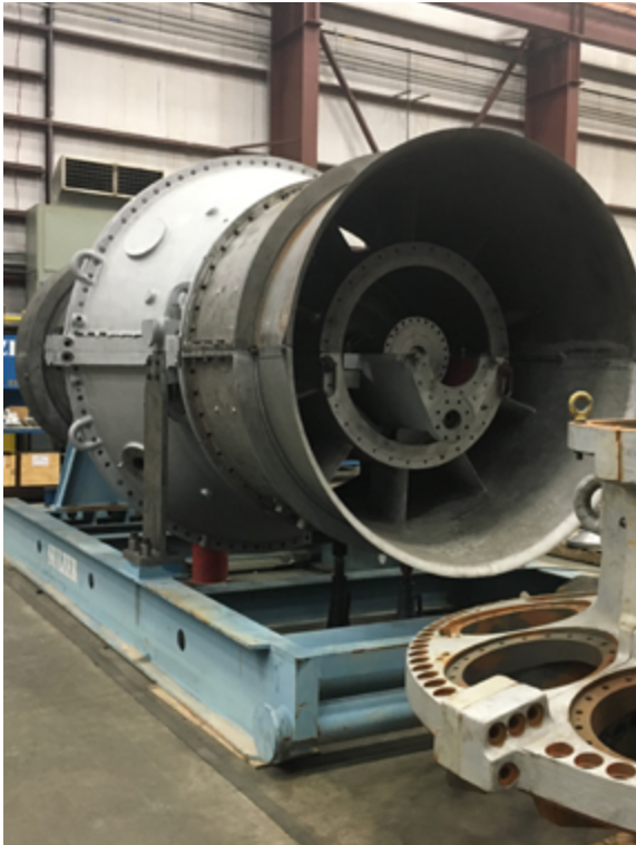
The original gas turbine thermal block was inspected and found to be beyond economic repair.
